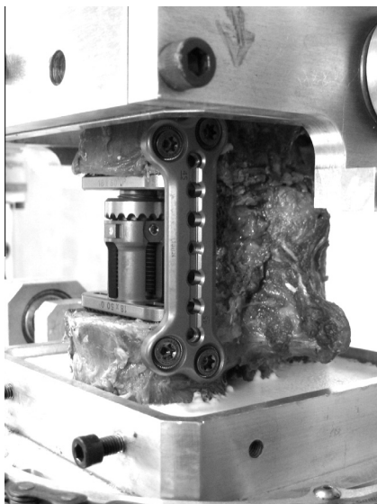
Fig. 1. Test construct showing T12–L2 spinal segments, L1 corpectomy, expandable cage with rectangular endcaps, and four-screw lateral plate.
