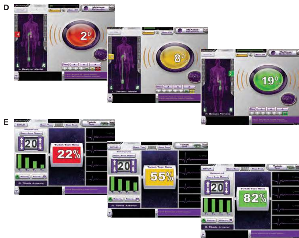
FIG. 8-8, cont'd D , The descending nerves of the lumbar plexus tend to lie in the posterior one third of the psoas muscle. The NeuroVision System assists with safe passage past these nerves and/or confirmation of their posterior location via evoked EMG monitoring. In Detection mode, the NeuroVision System continuously searches for the stimulus threshold that elicits an EMG response on the myotomes being monitored and audibly and visually reports the thresholds. As the Dilator is advanced through the psoas muscle, the stimulus necessary to elicit an EMG response varies with the distance from the nerve. For example, as the stimulus source moves closer to the nerve, less stimulus intensity is required to elicit a response, resulting in a lower threshold, which provides an indication of the relative proximity of the Dilator to the nerves. Literature reports suggest that stimulation thresholds of less than 5 mA may indicate direct nerve stimulation, 1-3 and other experience has suggested that threshold values greater than 10 mA indicate a distance that allows both continued nerve safety and ample working space. 4 E , The Twitch Test can be performed either in peripheral stimulation mode (the stimulation is directed through an electrode at the popliteal fossa) or direct stimulation mode (the stimulation is directed through instruments in the surgical wound). The system stimulates with four pulses and displays the results of each twitch as a percentage of the first one. A fourth twitch with at least 75% of the strength of the first is required to ensure accurately quantifiable EMG readings.
